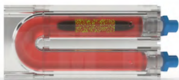
Figure 1) Demonstration of a bioreactor chamber with a black torpedo holder located on top of the bioreactor which holds the BMSC cell-seeded bio-scaffold.
